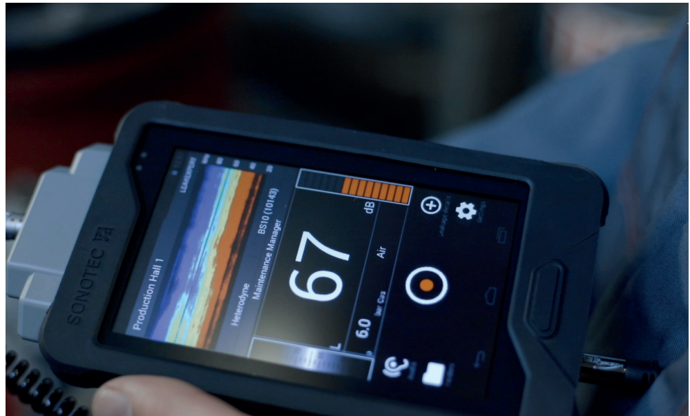
Leaks are broadband phenomena as the LeakExpert app on the SONAPHONE easily demonstrates
