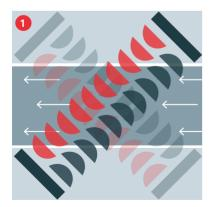
SONOFLOW flow meters use the ultrasound transit-time technology to accurately determine the flow rate. The sensor measures the time of flight of the ultrasonic wave with and against the flow direction of the liquid.
