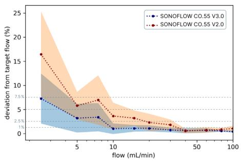
"Our latest non-contact clamp-on flow meter SONOFLOW CO.55 V3.0 combines accuracy and usability for low flow applications."
